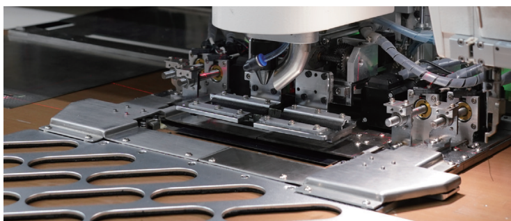
袋模长度可智能调节 The length of the pocket mold can be adjusted intelligently
